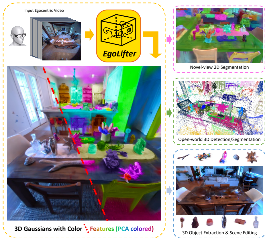
Fig. 1: EgoLifter solves 3D reconstruction and open-world segmentation simultaneously from egocentric videos. EgoLifter augments 3D Gaussian Splatting [16] with instance features and lifts open-world 2D segmentation by contrastive learning, where 3D Gaussians belong to the same objects are learned to have similar features. In this way, EgoLifter solves the multi-view mask association problem and establishes a consistent 3D representation that can be decomposed into object instances. EgoLifter enables multiple downstream applications including detection, segmentation, 3D object extraction and scene editing. See supplementary material for animated visualizations.
